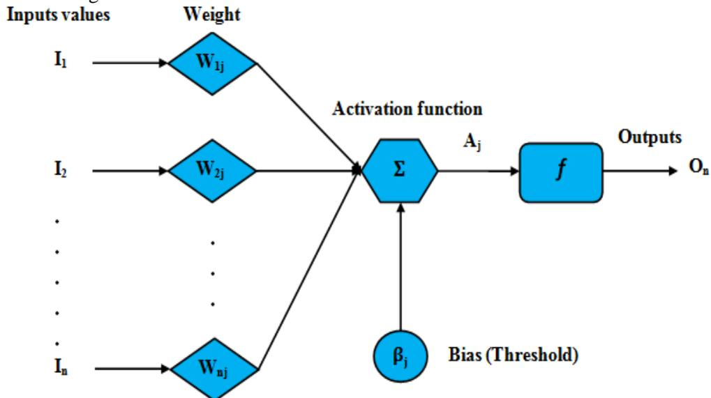
**Figure 3:** Structure of an artificial neuron.
