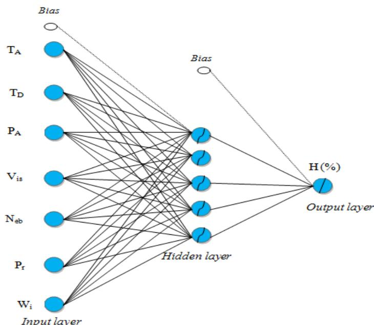
**Figure 9:** Architecture of the neural network to three layers of configuration {7-5-1} developed in this study.
